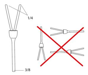
IMPORTANT: To ensure the same flow of refrigerant in every panel and consequently take advantage of the evaporation surface entirely; you should install the same tube length from the distributor to each panel. If a pipe is too long for the length require, it must be rolled up.
